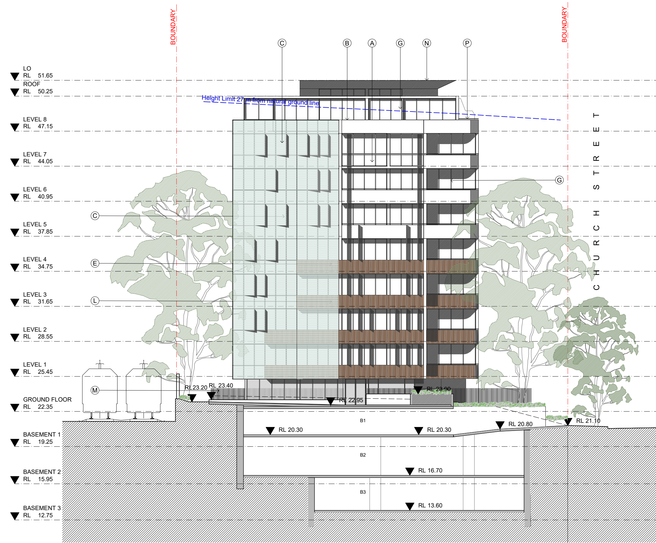
1 BUILDING D - EAST ELEVATION 1:200@A1
